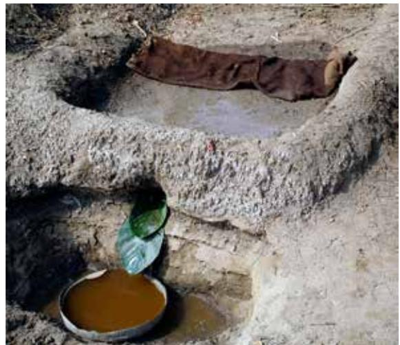
**Figure 15.** The extracted saltpetre liquor a being collected
