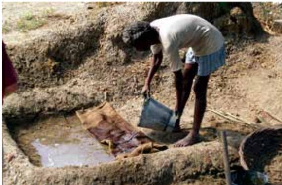
**Figure 14.** Pouring water over the saltpetre soil
