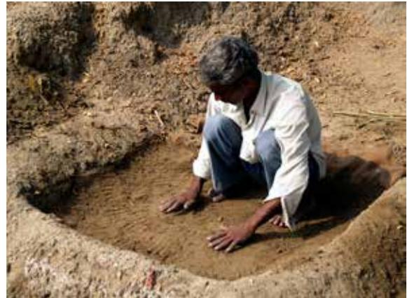
**Figure 13.** The saltpetre is carefully packed down
