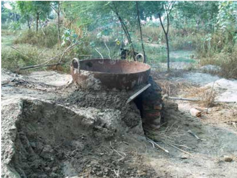
Figure 16. The pan for producing the crude saltpetre
