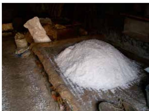
**Figure 26. The bamboo chali where the saltpetre is purified still further**
