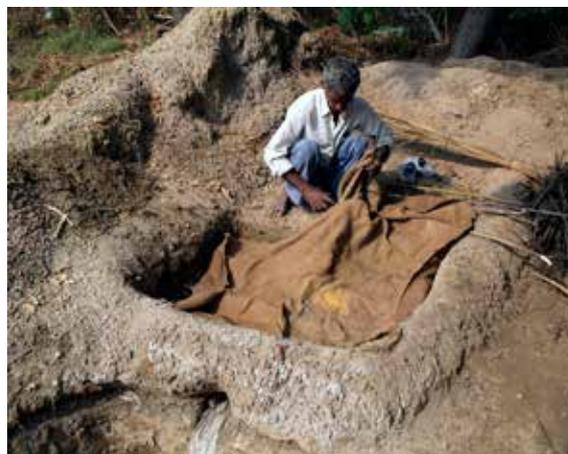
**Figure 11. Sacking is laid over the sticks**
