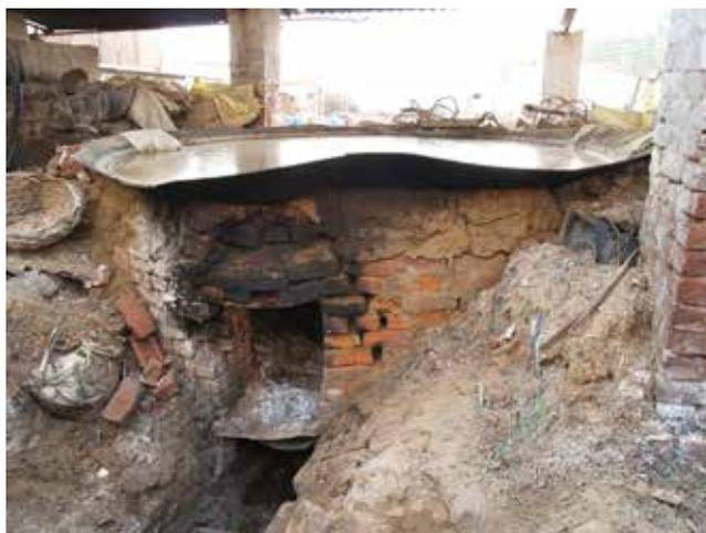
**Figure 9. The old iron pan at the second factory**
