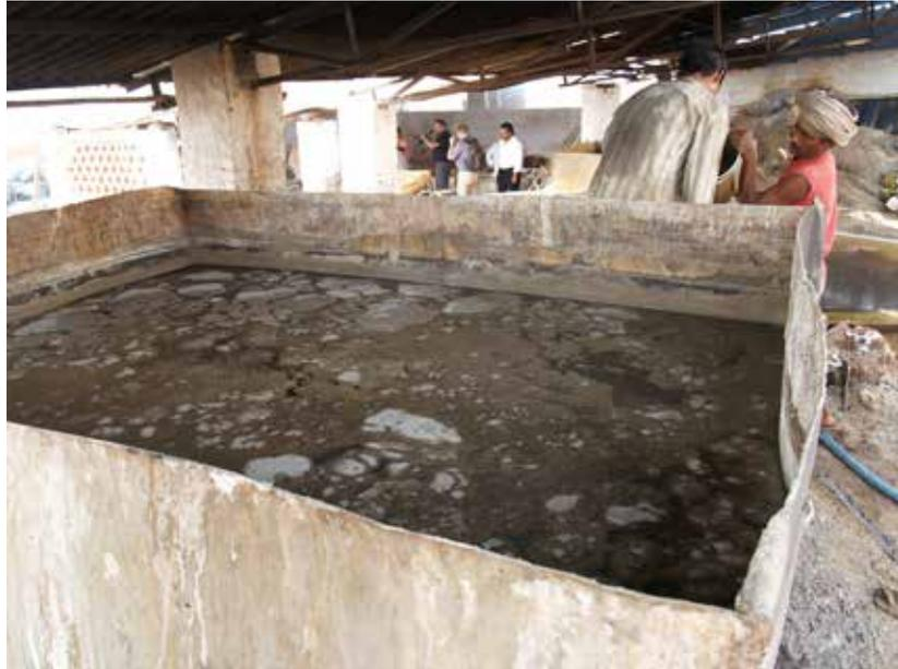
**Figure 4. The tank at the third factory containing the crude saltpetre from the first factory**
