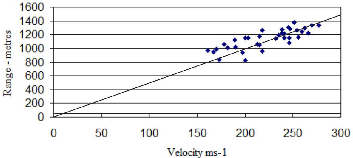
Graph of velocity versus range for the Loshult gun
