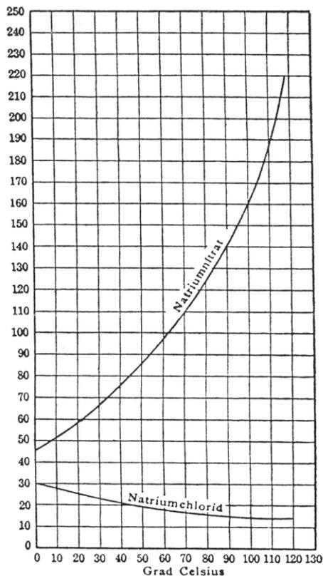
Figure 11 Solubility of a solution of sodium nitrate and sodium chloride
