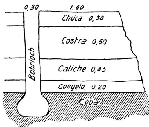
Figure 10 Cross section of 'saltpetre plateau' showing method of mining
